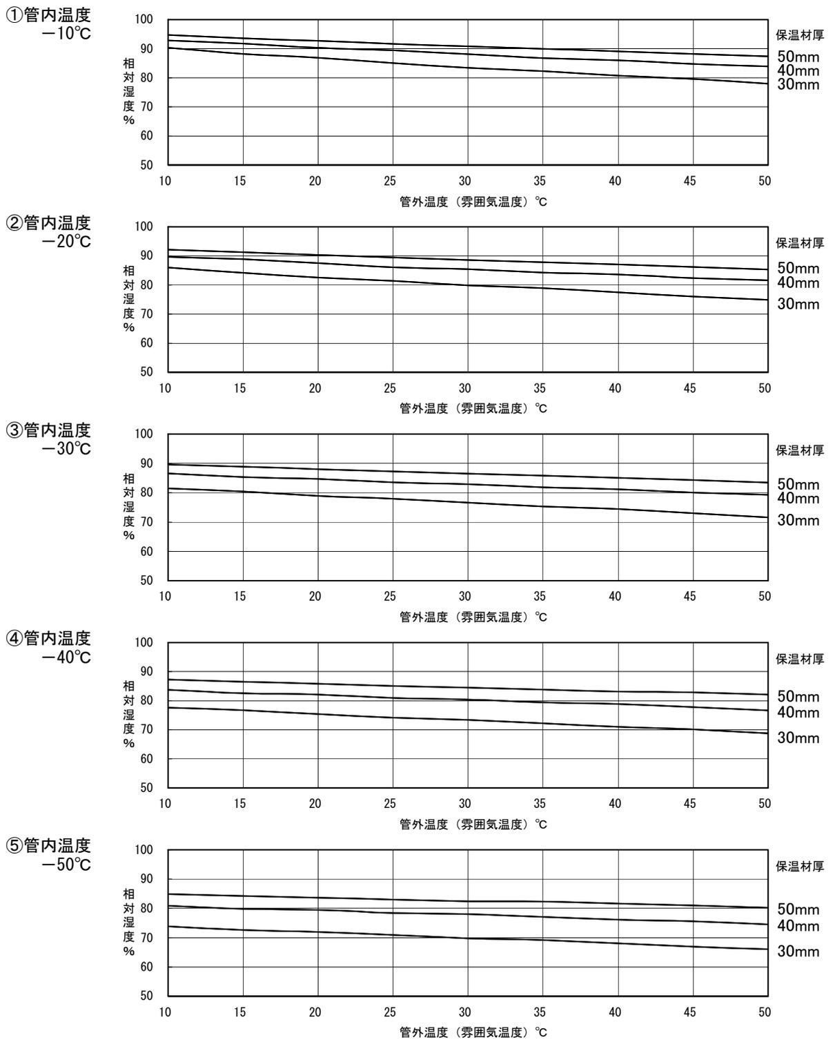
図-1 適合銅管  $\phi 15.88$
